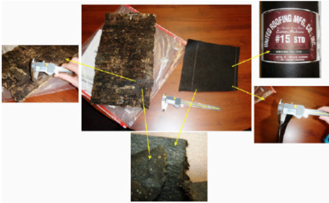
Figure 4: Comparison between Stock Type 1 #15 Felt and Apparent Building Paper on Exterior Side of Removed Section of OSB
